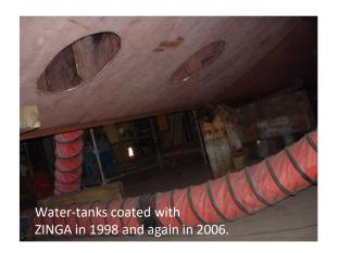
This yacht makes a ton of fresh water a day from her on-board desalination installation. The water tanks were originally epoxy-coated in 1998 when the yacht was built. But only six weeks later stray-current problems had caused cathodic disbondment of the epoxy coating, and it had blistered all over the tank walls with the subsequent rusting taking place. The problem with stray currents was sorted out and they were given a specification to apply ZINGA, which they did.
