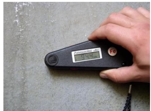
The surface of all metal structures was very rough and deeply corroded. The resulting surface finish after sand-blasting was very rough and uneven, all dappled with cavities, grooves, indents and pits. But all those indentations and cavities were cleaned up, blasted and coated with **ZINGA**.
