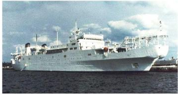
System: Blasting to SA 2,5 and Rz 50-70 µm ZINGA 1 X 100 µm DFT
