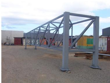
Surface preparation: Grit blasting to SA 2,5 and Rz 50-70µm
