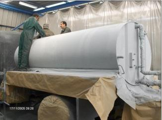
System: Surface preparation: Blasting SA 2,5
